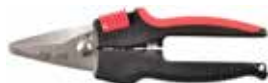
A Combinox, D50 The stainless steel blade cuts a wide range of material, and is notched for wire stripping. The spring opens cutter automatically with a thumb operated lock. Ergonomic handle with soft-insert.
